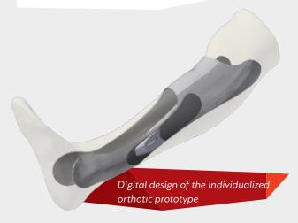
After post-processing, the .STL file is exported to CAD software, where a tightly fitting orthotic device is designed. The final step is to produce the orthosis using additive manufacturing. After the orthosis has been 3D printed, it is reinforced with carbon fibers and an epoxy composite.
