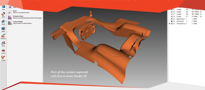
The car was 3D scanned in the owner's reception area and workshop; both areas had good stable lighting but no direct sunlight because this would affect the data capture. There were some dark carbon fibre areas around the wishbones – those were sprayed very lightly. Light reflections around the spoiler areas were also sprayed lightly to ease and quicken the capture. Paul recommends a few tips on how to capture car parts easier.
