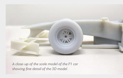
The car was surfaced at full size. Once it was scaled down, some of the thinner areas, in particular the wishbones and spoilers were thickened up in PowerSHAPE. The digital copy of the car was then 3D printed on Objet Eden 500V with a print layer of 0.016 mm.
