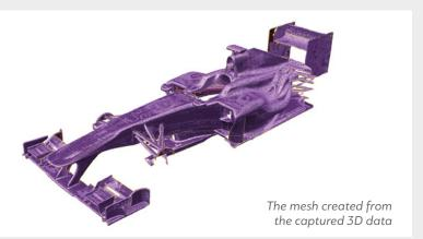
The completed 250 MB STL 3D model, approximately 8.5 million triangles, was then fully reverse engineered at Delcam using PowerSHAPE Pro. Complex doubly-curved regions were most suited to surface modelling, while more prismatic parts could be formed most efficiently using solids.
