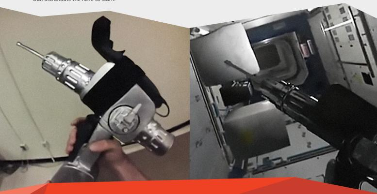
In 2015 NASA founded the Hybrid Reality Lab to combine consumer virtual reality technology and tracked 3D objects (locating an object in 3D space using object tracking technology) in order to make realistic visuals and tactile feedback, giving a much stronger and better sense of immersion.
